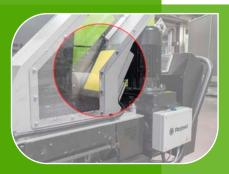
Metal detector, optional Hopper mounted metal detector – detecting metal in the hopper increases detection stopping the rotor before the metal reaches the cutter house. Detecting even embedded netal.
